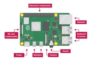
• Insert the SD card you've set up with Raspberry Pi OS into the microSD card slot on the underside of your Raspberry Pi.
