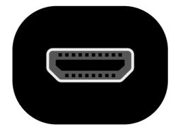
You need either a micro HDMI to HDMI cable, or a standard HDMI to HDMI cable plus a micro HDMI to HDMI adapter, to connect Raspberry Pi 4 to a screen.
